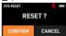
Enter this menu, select "CONFIRM", and press the confirm button to reset the device to factory settings. Resetting will only restore the device's system settings, and it will not erase the frequency data.
