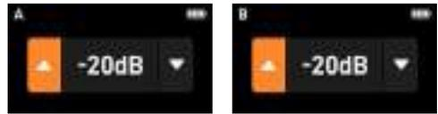
When the RX screen is on the home screen, a long press of the up button will enter the output gain adjustment page for audio output A, while a long press of the down button will enter the adjustment page for audio output B. You can use the up and down buttons to adjust the values for the output gain, with a range of -20 dB to +10 dB.
