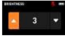
You can adjust the screen brightness across 5 levels. The configurable values are given as follows: (Dark) 1 2 3 4 5 (Bright). The default brightness setting is 5. Once adjusted, the system will retain your setting.
