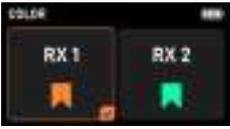
After entering this menu, you can choose a color label and synchronize the selected color to the paired TX, making it easier to distinguish devices that are paired and connected to the same frequency band.
